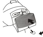
Reattach the lens and fasten the screws.
